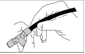
Cut off excess air line squarely. Install the air line into the fitting. This is a self–locking fitting. Push and slightly turn the cut end of the air line into the fitting as far as it will go. You will hear or feel a definite click when the air line is seated. Air line should go in  $^{9}/_{16}$ ". The air line is now installed.
