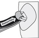
3) Pass the end of the webbing back through the open area of the two D-Rings on top as shown (3).
