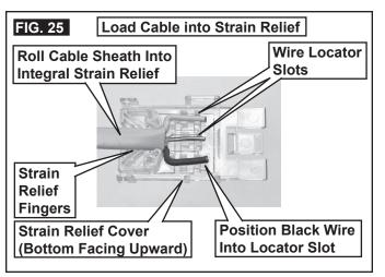
Lay wire into locator slots, making sure the black wire is placed into the polarization slot. See (FIG. 25). 8. Press the cable sheath into the integral strain relief slot. See (FIG. 25). Trimming of ground wire and possibly others will be necessary. Wires must not extend beyond the locators. See (FIG. 26).
