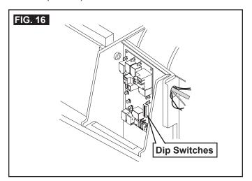
Dip switches are in the "OFF" position when shipped from the factory except heat pump and factory installed heat strip models. On these models the appropriate dip switch, heat pump or heat strip, is in the "ON" position from the factory.
