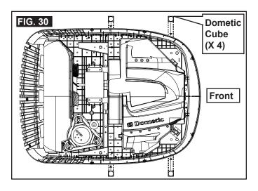
Maintaining alignment, place Dometic cubes beneath edge of base pan. See (FIG. 30), (FIG. 31) & (FIG. 32).
