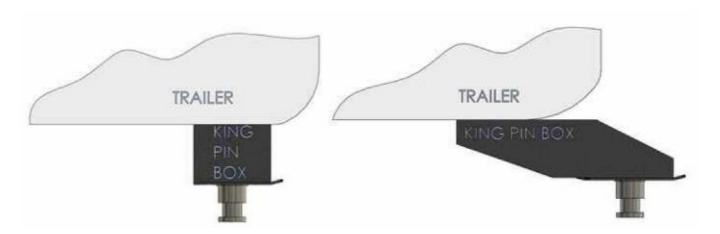
If the trailers king pin box is shaped like either of the above drawings there should be no problem adding the nine inch extension.
